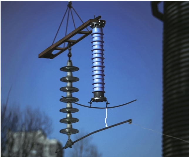
Figure 8. Testing of insulation protection capability against overlapping
